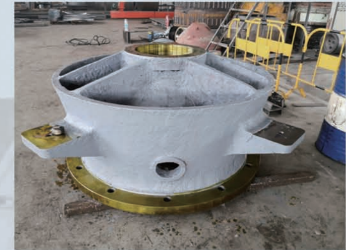
单液压缸圆锥破碎机下架体 Single hydraulic cone crusher lower frame
