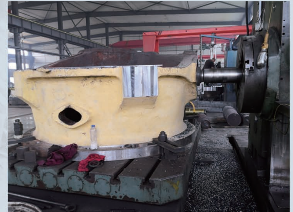
数控1.6米立车破碎机偏心套加工 CNC 1.6m vertical lathe crusher eccentric sleeve machining 数控4米立车单缸液压圆锥破碎机架体加工 CNC 4-meter vertical lathe single cylinder hydraulic cone crusher frame machining 数控160落地镗床圆锥破碎机架体加工 CNC 160 horizontal boring machine cone crusher frame processing
