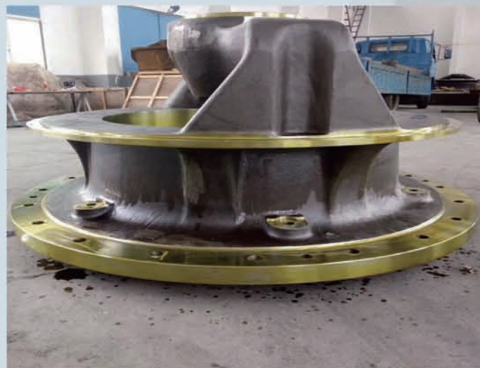
单液压缸圆锥破碎机上架体 Single hydraulic cone crusher upper frame
