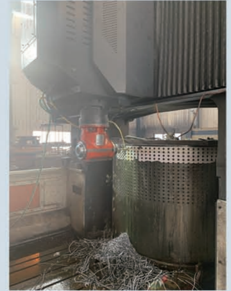
高压滚磨机辊套加工 High-pressure roller mill roll sleeve machining
