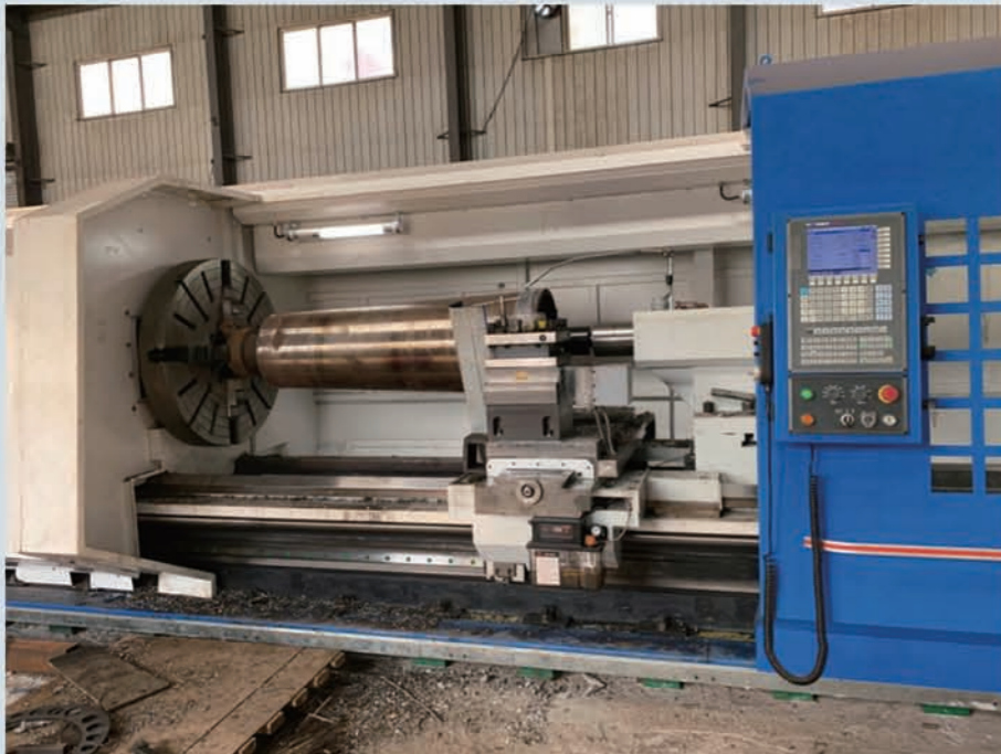
数控125全功能卧车 圆锥破碎机锥套加工 CNC 125 full-function horizontal lathe cone crusher taper sleeve machining
