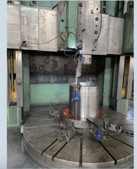
数控2.5米立车单缸500 偏心套加工 CNC 2.5m vertical lathe single cylinder 500 eccentric sleeve machining
