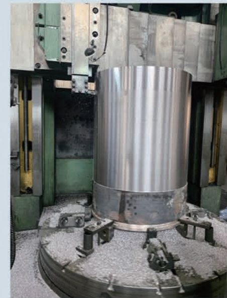
数控2.5米立车巡回 破碎机铜套加工 CNC 2.5m vertical lathe machining of copper sleeve of gyratory crusher
